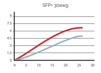
Lorom's noodl® cable assemblies provide a **40% to 75%** improvement in flexibility over industry standard cable assemblies. The above forcedeflection graphs demonstrate the force it takes to bend a given length of cable at a certain distance. The slope of these force-deflection curves is equivalent to the perceived cable flexibility.
