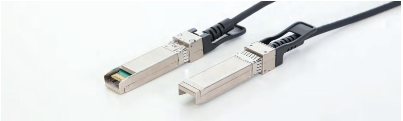
SFP+ passive copper cable assemblies provide a low cost alternative to fiber modules for short reach applications. They address applications such as 10 Gigabit Ethernet and 16G Fibre Channel. For these applications they support bidirectional serial data transmission rates from 1.125 Gbps to 14.025Gbps.
