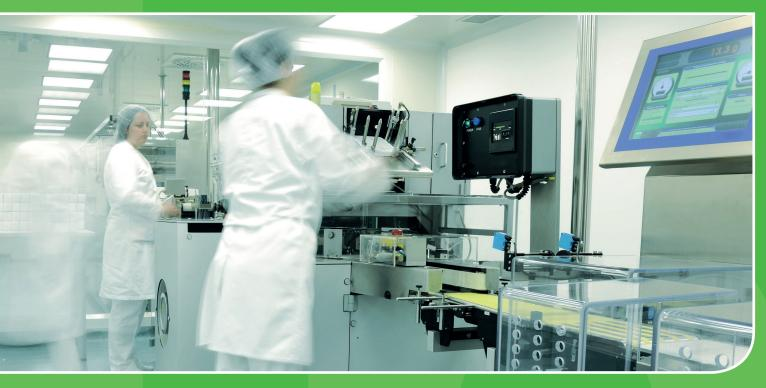
Our manufacturing facility features an ISO 8 (equivalent to GMP requirements 100,000) 600 m2 Clean room assembly area which meets China Standard YY0033-2000, our clean room is Bio burden monitored and controlled.
