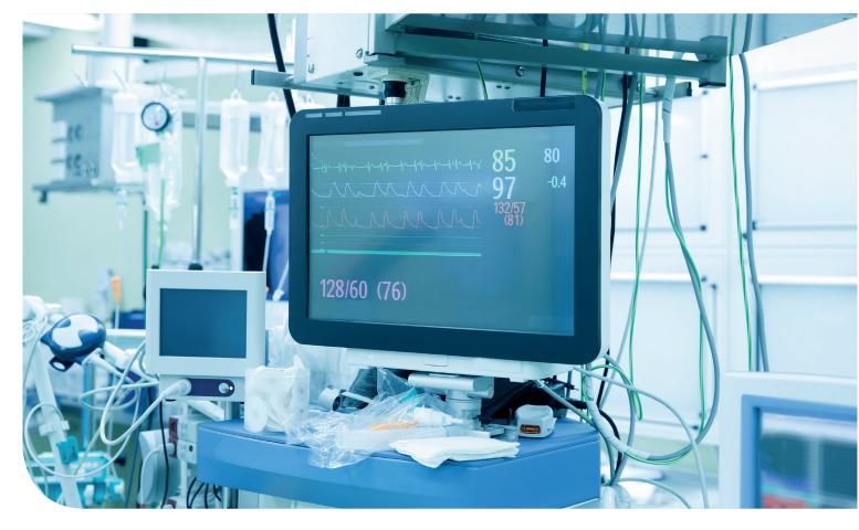
Patient Monitoring cable assemblies transmit signals from electrodes or sensors placed on the patient's body to the monitoring instrument that processes the signals.
